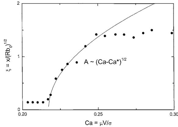
Fig. 2. Evolution of the dimensionless amplitude of the deformation of the interface as observed vs. the capillary number in the case of a Newtonian fluid (glycerol/water solution,  $\mu = 105$  mPa s,  $\sigma = 54$  mPa m) for a gap  $b_0 = 0.4$  mm and fitted by Eq. (1), with  $\alpha = 0.5$ .
