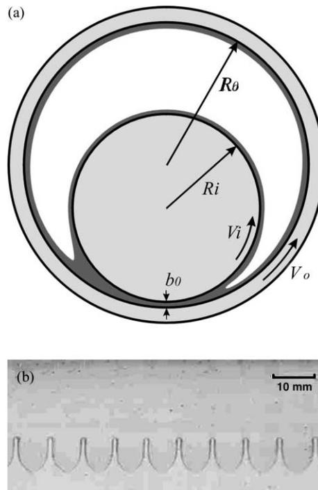
Fig. 1. (a) Sketch of the two-roll setup.  $R_i = 33$  mm,  $R_o = 50$  mm. Roll spacing  $b_0$  can be adjusted with a precision of 0.01 mm; (b) picture of the meniscus above threshold for a 1000 wppm Xanthan solution. Air is on top, and the bottom line corresponds to minimum gap position ( $b_0 = 0.4$  mm,  $Ca = 0.38$  and  $V_i = 160$  mm/s).
