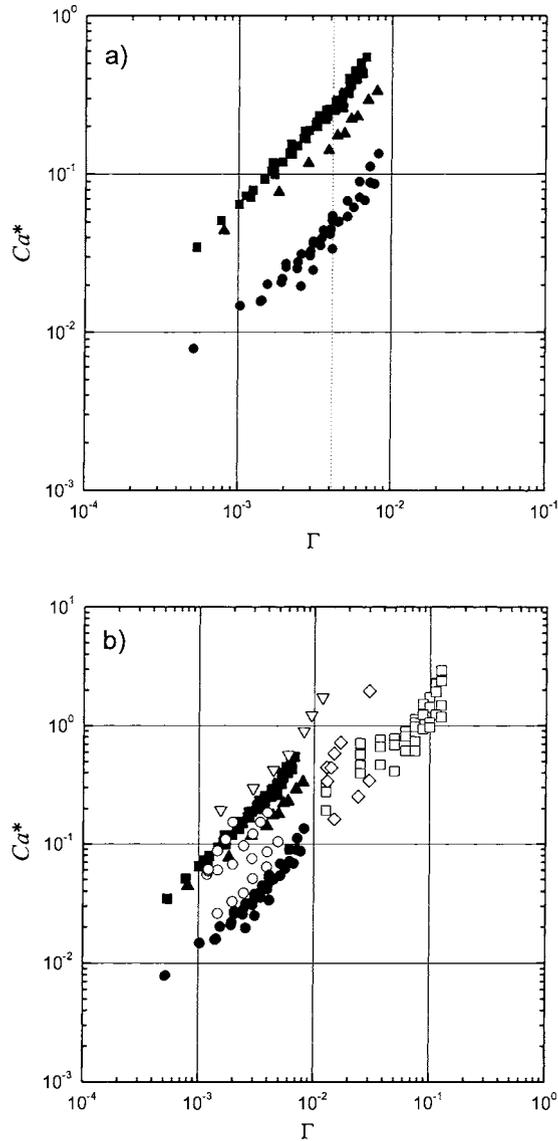
Fig. 6. (a) Log–log plot of the threshold value  $Ca^*$  vs. the aspect ratio of the cell  $\Gamma$ . (■) Newtonian solvent; (▲) Xanthan solution 2000 ppm; (●) PAAM solution 3000 ppm. Dotted vertical line corresponds to  $\Gamma = 4.12 \times 10^{-3}$ , the value at which critical  $Ca^*$  vs. polymer concentration has been measured (Fig. 7); (b) comparison between our data (filled symbols) and (□) [21]; (○) [20]; (◇) [18] and (▽) [24].
