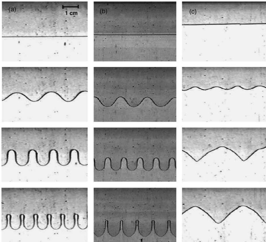
Fig. 8. Pictures of the interface below and above threshold (increasing  $Ca$  from up to down). On each picture, air is on the upper side. Minimum gap  $b_0$  is exactly located at the lower boundary of each frame ( $b_0 = 0.4$  mm). (a) Glycerol solution ( $Ca = 0.210, 0.226, 0.262, 0.425$ ); (b) Xanthan 1000 wppm ( $Ca = 0.076, 0.123, 0.155, 0.338$ ); (c) PAAm 1000 ppm ( $Ca = 0.110, 0.124, 0.154, 0.165$ ).
